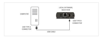
Connect the Local Extender into your computer using the included USB 2.0 cable
