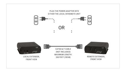
Connect the power adapter into your desired unit—Local Extender or Remote Extender.
