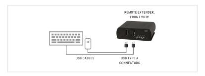
Attach your USB device(s) to the Remote Extender
